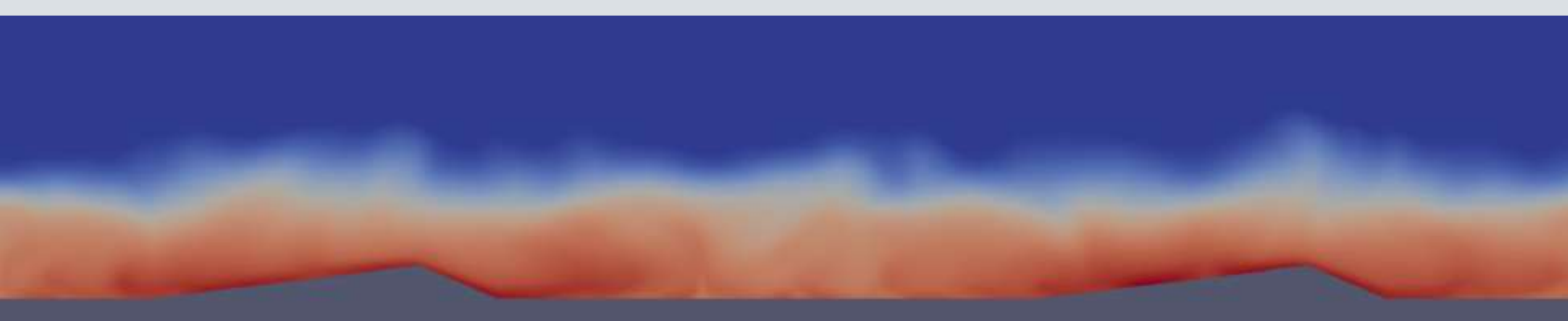
Figure 2: Sand transport over rippled bed simulated with mixtSedFOAM
